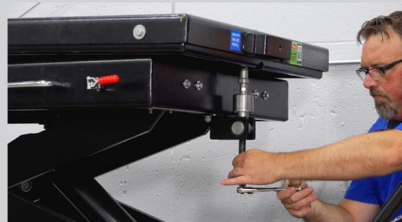
Adjust the tabletop with the object being removed or installed +3°/-1°. Tighten to raise the side with the tilt mechanism and loosen to lower it by using a 14mm or 9/16" socket or wrench.
