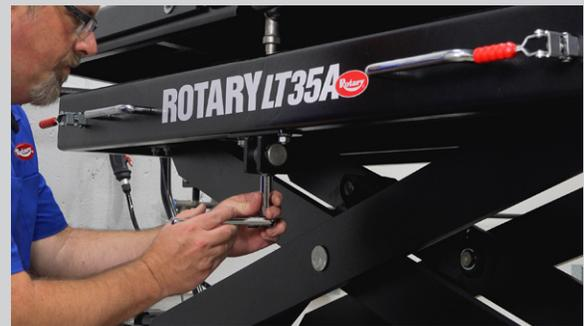
Use a 14mm or 9/16" socket or wrench on tilt mechanism located on the right side of the lift table to raise or lower platform +/-3°.
