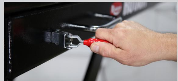
For fine platform positioning, release the four red-handled swivel locks on both sides of the lift table allowing the tabletop to move freely. Re-engage locks when fine positioning is not needed.
